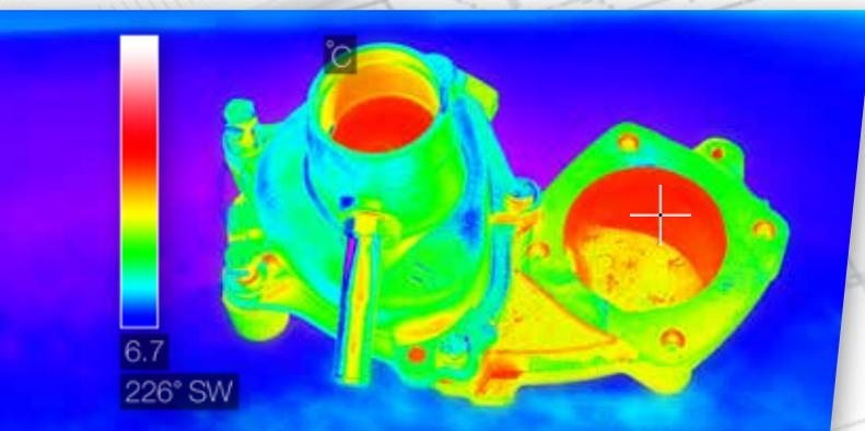
The endurance test bench is a standard 1000 hr endurance test where the spindle bearing is assembled into a specific Comline water pump reference, then attached to a test rig simulating the action of a real engine. Within this test rig coolant set at a constant 90°C is circulated by the prototype water pump. Each new-to-range Comline water pump reference undergoes this endurance test for a duration of 6 weeks.
