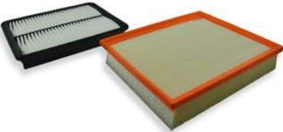
The air filter features a moulded, **Polyurethane (PU) or Polypropylene (PP) frame** designed to provide structural support and maintain filter media integrity. Selected PU and PP applications are supplied with a pre-filter layer, usually foam, designed to capture larger particles such as dust and soot. In dry, dusty conditions pre-filters are particularly useful in protecting filter media and help maintain filter performance.
