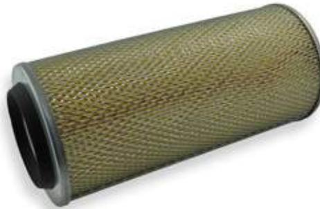
Visually a metal filter can look the same as a PU or PP variant, the crucial difference is that structural support is provided by a **metal, typically steel, frame** as opposed to moulded plastic. Such filters are mainly used within the Japanese and Korean vehicle parc.
