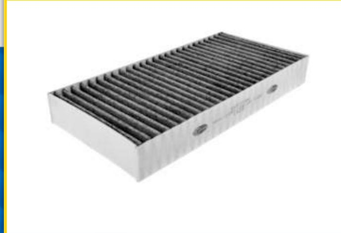
Alongside a range of cabin filters Comline also offers **activated carbon** options which offer an added layer of protection. The design of a carbon filter sees the media impregnated with activated carbon molecules that filter out harmful, ultra-fine gas particles such as Benzene or Ozone, plus absorb unpleasant odours which may otherwise enter the vehicle cabin.
