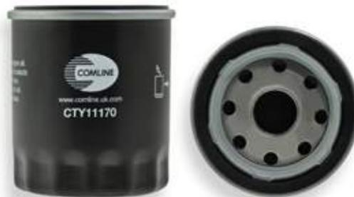
The **spin-on oil filter** takes its name from the process used to fit this type of part, where the entire filter, including housing, is quite literally 'spun on' to the vehicle's oil system. Spin-on filters are self-contained within a metal canister meaning the filter media, bypass and anti-drain valve, element cover and gasket are all built into the design.
